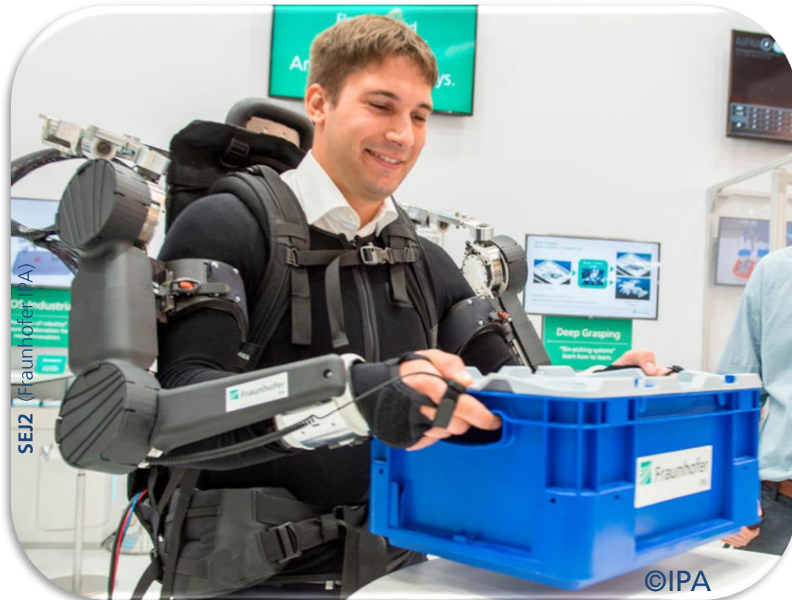
ExoJacket: Fraunhofer IPA – Research active Exoskeleton demonstrator for upper body support and protection
